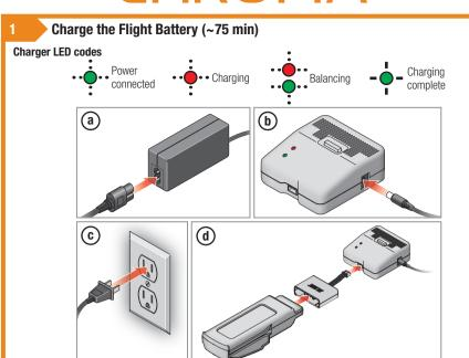
CAUTION: All instructions and warnings must be followed exactly. Mishandling of Li-Po batteries can result in a fire, personal injury and/or property damage.
