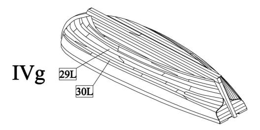
h) Glue second planking 31 to the hull. Glue the planks in direction from stem to stern.
