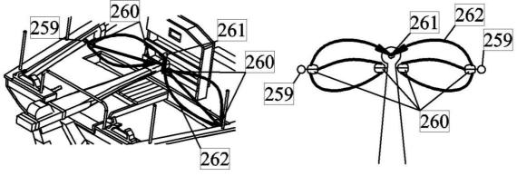
c) First glue windlass VIIc to the bow. Then glue also other parts to the bow as it is shown in the figure. Finally drill a hole for bowsprit.
