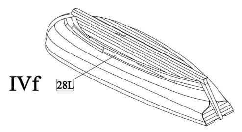
g) Glue second planking 29 and 30 to the hull. Glue the planks in direction from stem to stern.
