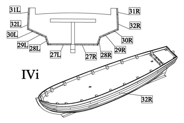
i) Glue second planking 32 to the hull. Glue the planks in direction from stem to stern.
