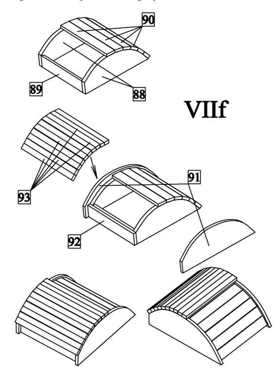
f) First glue skeleton from parts 88-90. Then glue parts 91-93 to the skeleton.
