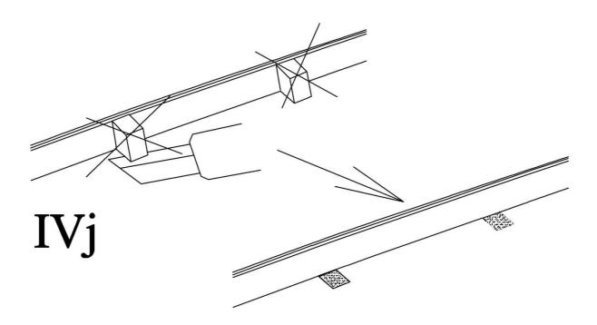
k) Glue from parts 33-36 steering post if you're building the sailing version and then glue it into to hole in the deck as it is shown in the figure.
