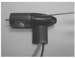
2. Connect the center body fairing to the back of the motor using the two 2mm x 5mm screws provided. Note: You may want to trial fit the center body fairing so you can make sure the wires are accessible to plug into the ESC when the motor is attached to the fan unit. You may have to re-position the fairing before attaching to the motor.
