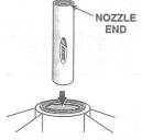
INSERT ENGINE INTO REAR OF BOCKET
