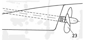
9. Parts 21 to 28. Carefully drill the hull to accept the prop shaft, use an undersize drill and file to fit. Insert the shaft and tube and with the motor in position coupling 26 as an aligning jig to ensure complete accuracy.
