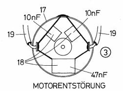
Then refer to drawing 3. Solder on the motor wires and suppression capacitors. Screw the motor to the mount with the screws provided.
