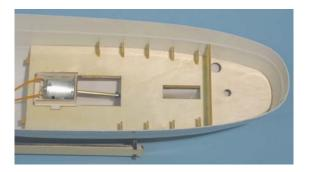
Carefully drill pilot holes for the motor mount screws and screw the mount in position. When fixed Epoxy glue the shaft and support 28 in position.
