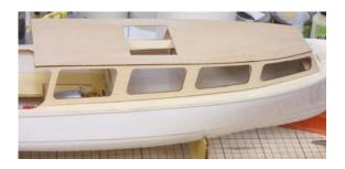
Drill the roof for the hand rail supports 54 fix these in position allowing a 2 mm gap from the roof. Fit and glue the hand rail 55.
