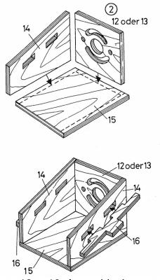
8. Parts 12 to 16. Assemble the motor mount as shown on drawing 2.
