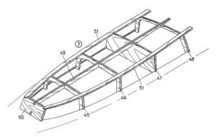
14. Parts 45 to 55. Assemble the cabin frame as shown in drawing above.
