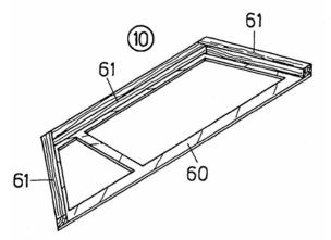
16. Parts 60 to 65. Construct the bridge as shown on the main drawing and drawing 10. Leave the bridge in a natural, wood finish. Paint the roof to match the Cabin roof.
