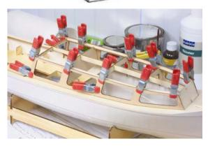
Fix the roof to the cabin. When dry cut out the roof as marked and also remove the centre spar. Paint the cabin, inside and out to your chosen colour scheme.
