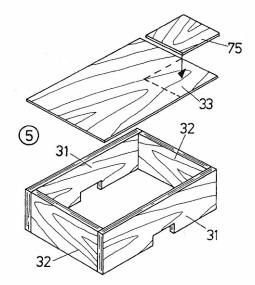
Assemble the engine room cover as shown in drawing 5. Part 75 door step panel can be fitted later after painting.
