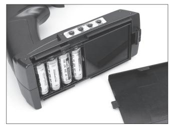
Install a fully charged 7.2V Ni-MH battery pack into the radio box. Follow the instructions included with your fast charger to ensure a safe charge. Plug the battery into the female battery connector attached to the electronic speed controller.
