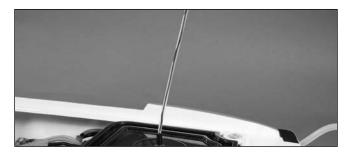
The rudder control arm should move toward the front of the boat when right input is given. Conversely, when left input is given, the control arm should move toward the back of the boat.
