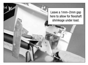
3. Lubricate the drive shaft with PRB0100 Waterproof Marine Grease (see your local hobby shop). Reinstall the drive shaft in reverse order. Be sure to reinstall the nylon washer between the universal and the stuffing box.
