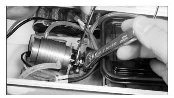
2. Remove the 3mm propeller strut screw and remove the drive system by sliding the flex shaft out of the stuffing box.
