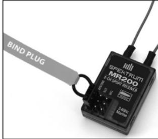
2. Power the receiver through any open port. The LED on the receiver should be flashing, indicating the receiver is in bind mode and ready to be bound to the transmitter.
