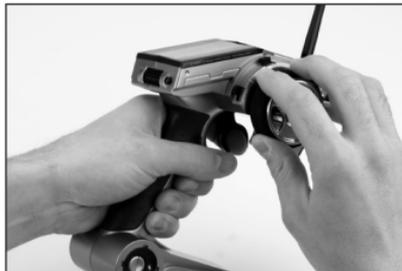
4. Follow the procedures of your specific transmitter to enter bind mode; the system connects within 15 seconds. Once connected, the LED on the receiver will go solid indicating the system is connected.
