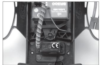
Once the battery is charged, remove the body clip from the front battery hold-down and lift the battery strap.
