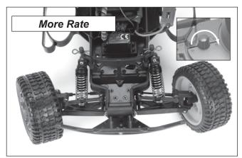
For sharper or additional steering, try turning the knob clockwise (to the right).
