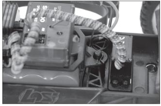
Reinstall the battery strap and body clip. Plug the battery pack into the ESC.
