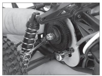
When adjusted properly, you should be able to hold the rear tires firmly and barely be able to push the spur gear forward with your thumb.
