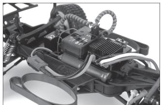
Install the charged battery pack into the chassis as shown. Ensure the battery is laying flat on the chassis.
