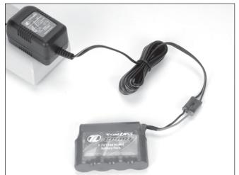
Plug the charger into the proper wall receptacle then the battery into the charger and let it charge for 3 hours for the first time. For subsequent charges allow 5 to 6 hours for a full charge.
