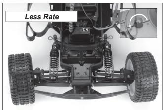
If your Mini SCT turns too sharply and/or spins out easily, try turning the steering rate down by rotating the knob counterclockwise (to the left).
