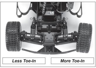
Ideally, you want the front of the tires to be pointed inward toward each other just slightly when viewed from above. This makes the model track straight and stable. This is controlled with the threaded steering rods on either side. As you make them longer you will increase the toe-in and vice versa.
