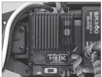
Once the transmitter has been powered on, turn on your vehicle by sliding the switch on the ESC to the "ON" position.
