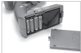
Remove the transmitter battery cover, install four (4) AA batteries and replace cover. Pay close attention to the polarity of the positive (+) and negative (-) ends and replace cover.
