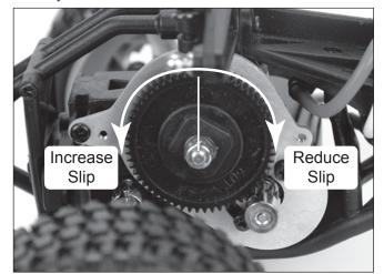
Adjustment is made by turning the 3mm adjustment nut clockwise (to the right) to reduce the slip, or counterclockwise (to the left) to increase the slip.
