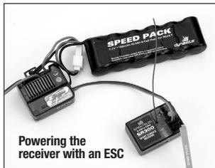
Powering the receiver with an ESC
